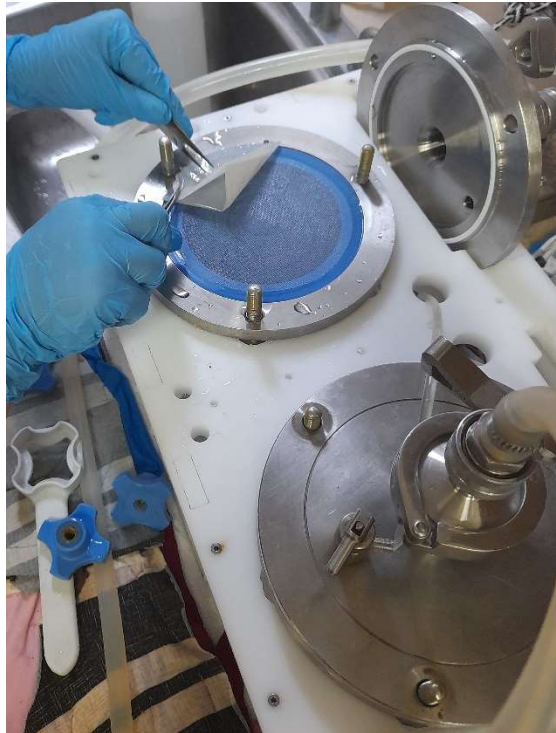
Filter recovery following seawater filtration using customized unit containing special filter holders and a peristaltic pump. Photo: Ophelie Choupin.
