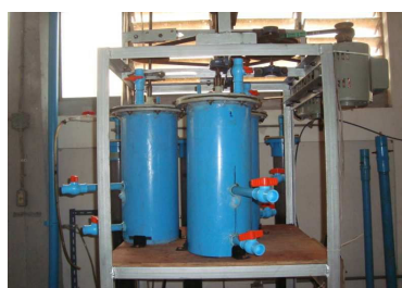
Fig. 2 the anaerobic reactors
