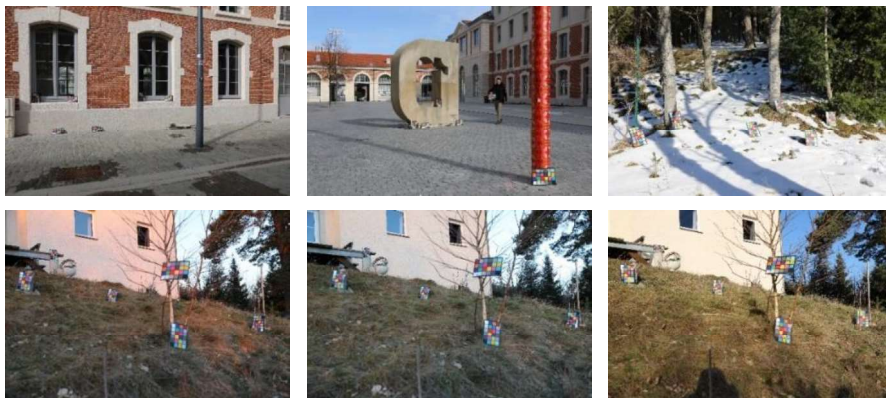
Figure 5: Outdoor images captured with the same Canon camera, taken under multi-illuminant conditions (eg. shadows, daylight shifts, etc.). In each image six color charts were put in various positions and distances to the camera.
