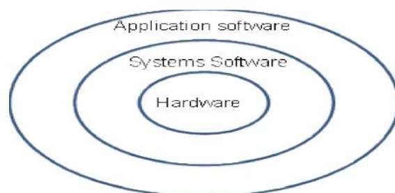
Fig. 1 Relationship between hardware, system software and application software[4]
