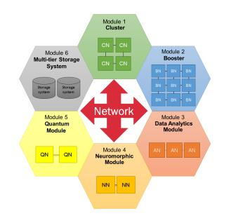
Fig. 1. Schematic representation of Modular Supercomputing Architecture.
