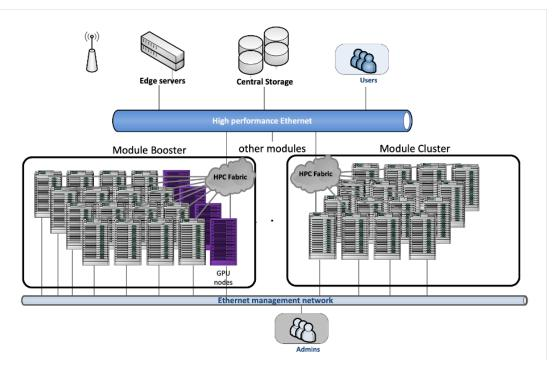
Fig. 2. Network architecture of a Modular Supercomputing Architecture.
