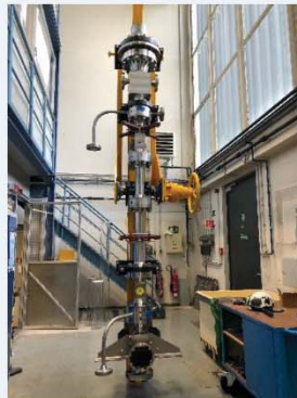
Figure 1: First trial setup of the COSMOS-H test track in McSAFER
