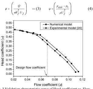
Fig. 3 Validation characteristic curve of Head coefficient vs. Flow coefficient.
