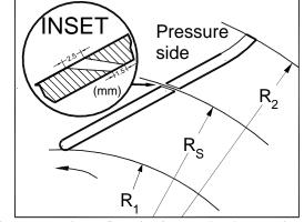
Fig. 4 Geometric Configuration for Boundary layer suction slot provided on the Impeller
