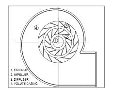
Fig. 1 Model of the centrifugal fan used in the analysis.
