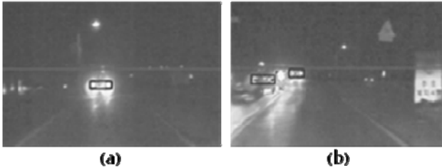
Fig. 4 Result of classified vehicle's pair lamp light. (a) one vehicle's lamp light classify, (b) many vehicles' lamp light classify.
