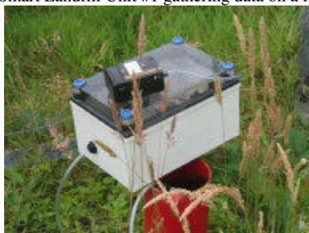
Figure 5 Smart Landfill Unit #1 gathering data on a field trial
