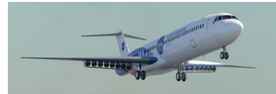
NASA SUZAN Distributed propulsion + BLI tail-fan
