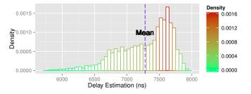
Fig. 3. One-way delay profile considering concurrent in-line fronthaul stream carrying 16 CPRI BFs of 128 bits per frame.
