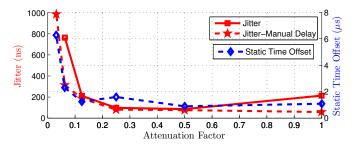
Fig. 4. Jitter and static time offsets for varying attenuation factors.
