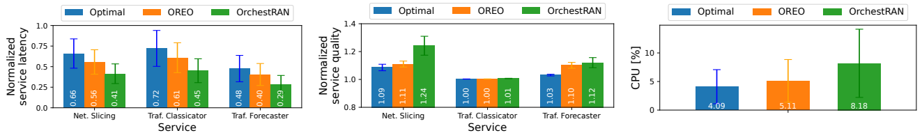
Fig. 7. Testbed results: normalized service latency (left) and quality (center), and CPU consumption (right) of OREO, Optimal and OrchestRAN.
