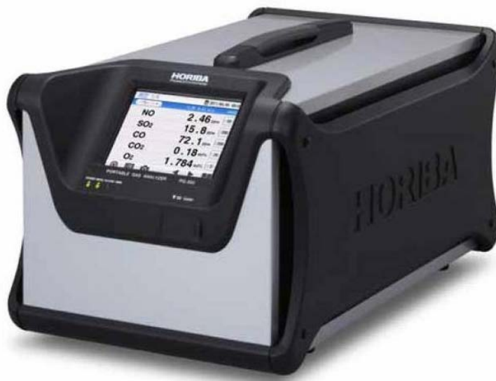
Figure 9. Horiba PG-350 Gas Analyzer [43]
