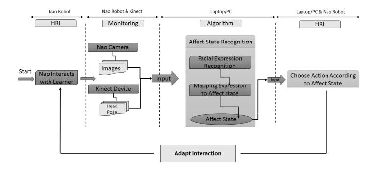
Fig. 1. A full cycle of our framework. Nao robot begins interaction with the learner, e.g., a learning task. Robot's camera and Kinect device inputs the affect recognition algorithm with images of the learner and her/his head pose respectively. The algorithm outputs the affect state of the learner and the robot decides for its next action accordingly.
