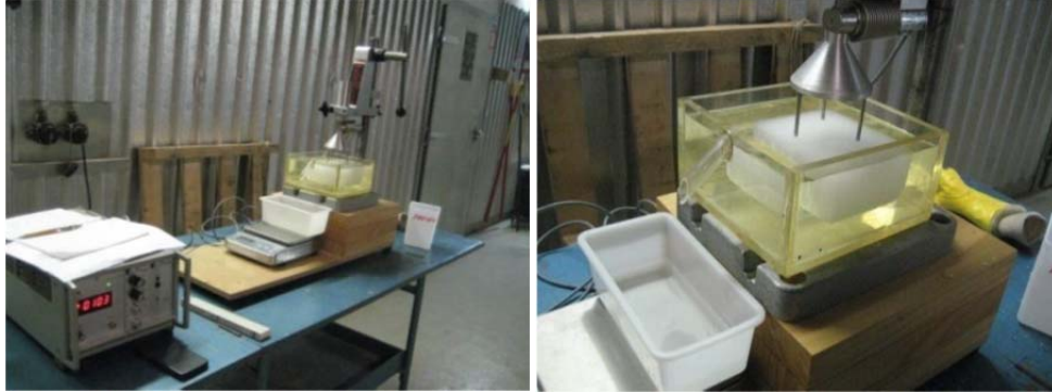
Figure D4. Test setup for ice density tests at HSVA
