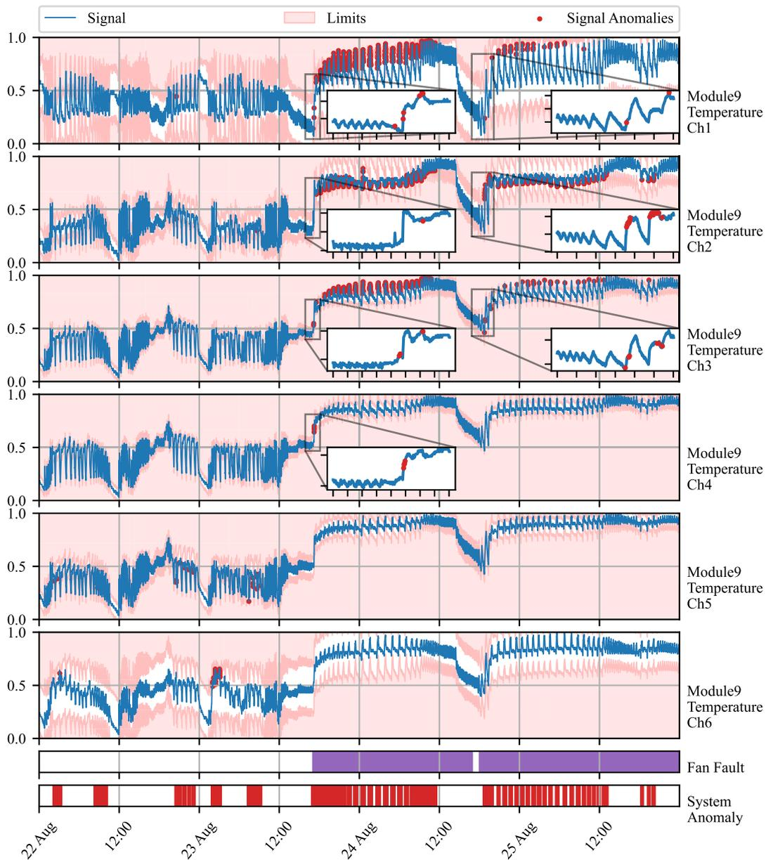
**Fig. 10.** Time series of battery module 9 measurements (blue line). The  $y$ -axis renders the normalized deviations of temperature from the average of all modules. Signal anomalies are marked as red dots. The light red area represents an area out of dynamic operating limits. True fan faults are marked by purple bars. Green bars represent the times of changepoint detection. Red bars denote the period where any signal anomaly.
