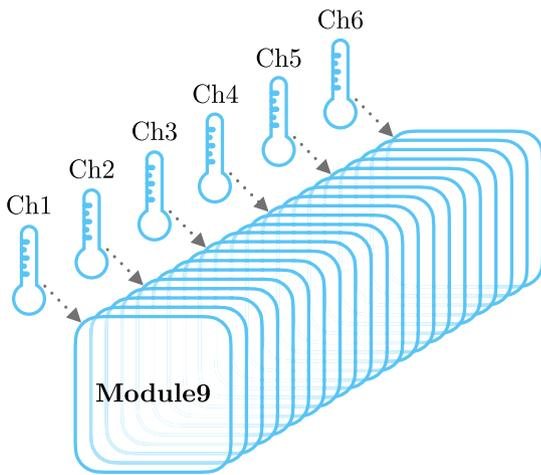
**Fig. 9.** Module 9 with 20 cells and 6 sensors measuring the temperature at each 4th cell.
