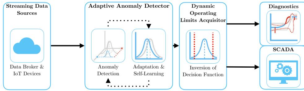
Fig. 1. Schematic representation of the proposed method AID.
