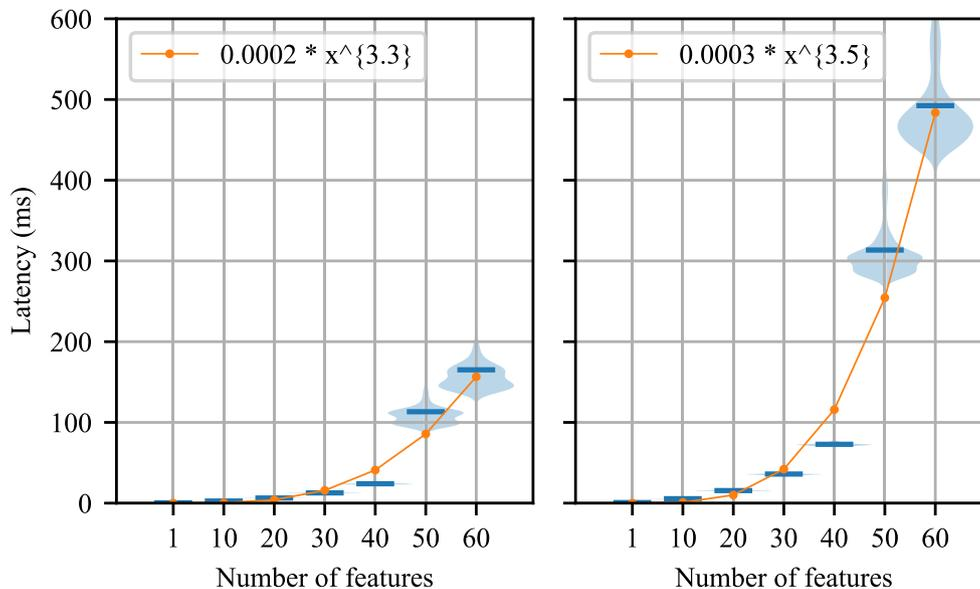
Fig. 12. Analysis of latency distribution of the proposed method AID. Violin plots depict the distribution of the latency for varying number of features, while horizontal bars show mean latency.
