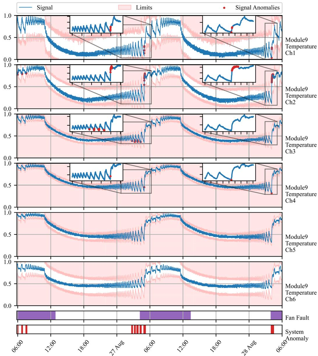
Fig. 11. Time series of battery module 9 measurements (blue line). The y-axis renders the normalized deviations of temperature from an average of all modules. Signal anomalies are marked as red dots. The light red area represents an area out of dynamic operating limits. True fan faults are marked by purple bars. Green bars represent the times of changepoint detection. Red bars denote the period where any of the signals contained anomaly.
