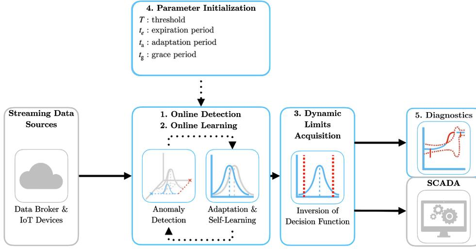
Fig. 3. Schematic representation of the proposed method AID with parameter initialization. Colored boxes represent steps described within the subsection.
