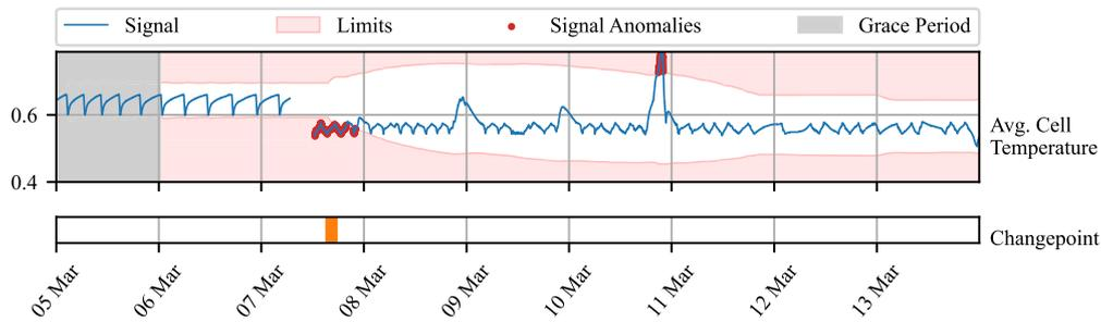
Fig. 6. Detection of anomalies using model **with** adaptation to change points over the same historical measurement as in Fig. 5. The change point is detected  $t_a$  hours after the anomaly is alerted, triggering adaptation to changed behavior more than two days sooner, compared to model **without** adaptation to change points in Fig. 5. The adaptation is reflected in changes in dynamic operating limits. The system alerts anomalies for approximately 10 h.
