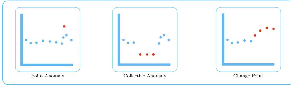
Fig. 2. Illustration of sample scenarios of point anomaly (measurement with significant dissimilarity), collective anomaly (cluster of abnormal points), and change point (initial sequence of changed operation) detection.
