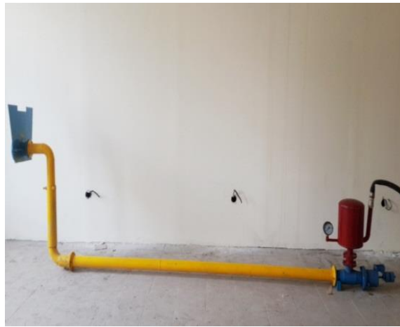
Pic. 2. General view of the GNU - 5-15 hydraulic ram pumping unit of the KazNARU design (option 1)
