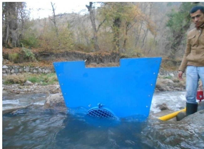
Pic. 3. Fragment of tests of the GNU - 5-15 hydraulic ram pumping unit of the KazNARU design (option 1)
