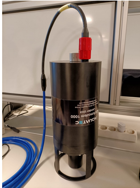
Figure 15: AQUATEC Acoustic modem.
