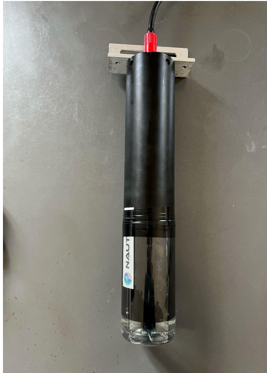
Figure 5: NIVA's pH sensor.
