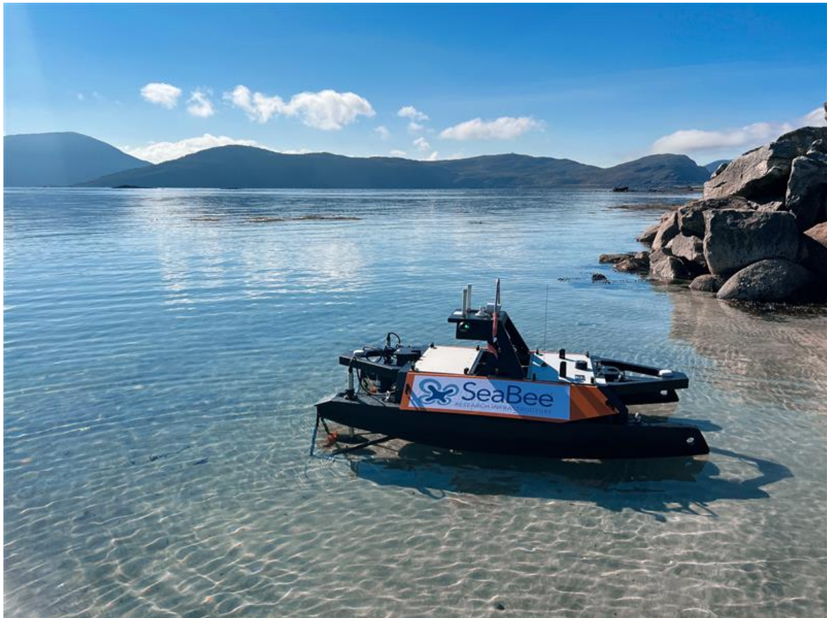
Figure 3: Otter ASV Platform provided by NIVA.
