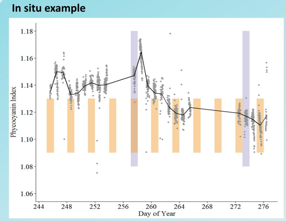
Intra-daily and daily variations of cyanobacteria pigments in Mantua Lakes (Lombardia Region, Italy) based on spectral indexes obtained by operating an autonomous spectroradiometer in the field for about 30 days (Hestir et al. 2015)
