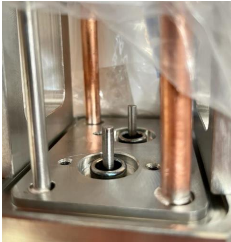
Figure 4.5. RF feedthroughs TIG welded to ion source flange
