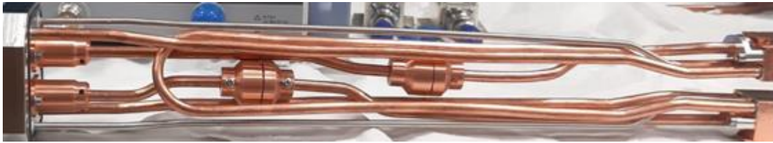
Figure 4.7: Intermediate connections mounted at each of the coaxial cable lines of the ion source
