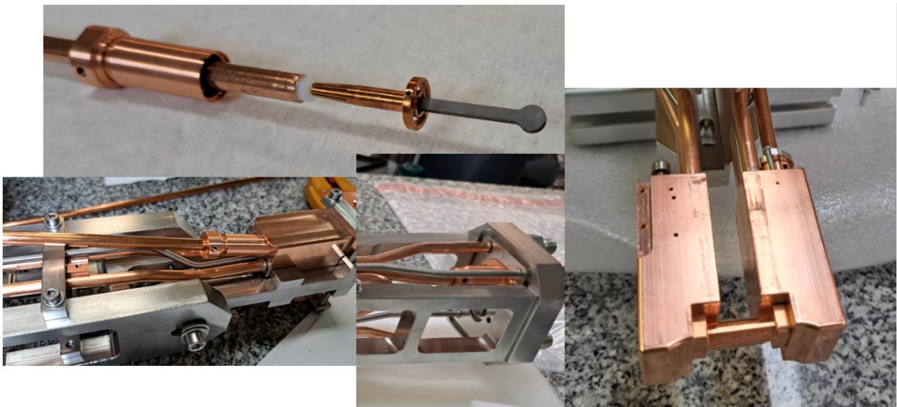
Figure 4.6: Images of some of the assembly steps. Cathode – RF window – coaxial cable -copper connector assembly (up-left), insertion of that structure into the ion source main body (bottom-left), connection of the other side of the coaxial cable to the RF feedthrough at the flange side (bottom-center), assembly of the chimney (right)
