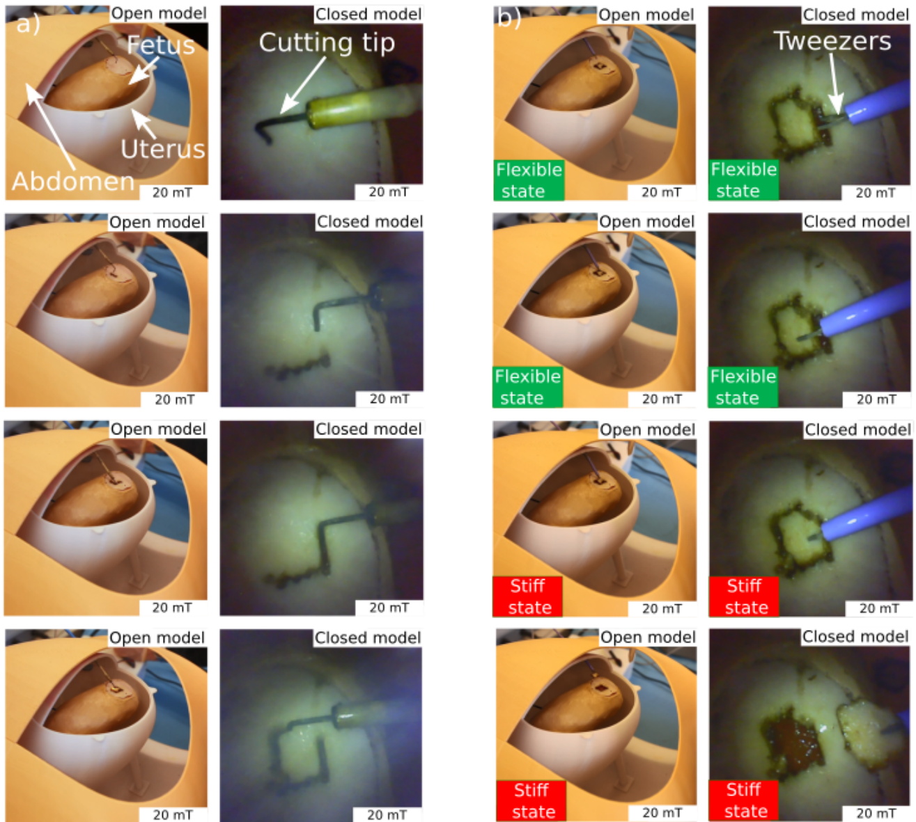
Fig. 5. Experimental defect resection. a) Sequence showing the monopolar catheter cutting the porcine flesh disc. In the left column, the experiment is demonstrated by opening one panel of the abdomen model. In the right column, the experiment is demonstrated using only the camera catheter view with the abdomen model completely closed. The catheter was guided in a rectangular pattern using the external magnetic field. For this experiment, the monopolar catheter was set to a cutting power of 150 W. The high power produced a small amount of smoke when the experiment was conducted in the completely closed model. b) The severed porcine flesh rectangle was removed using the tweezers catheter. The catheter was initially in the flexible state. In this state the VS section is flexible and allows the catheter tip to be guided towards the skin to be removed. When the tweezers tip was within grasping range, the VS module was switched to the hard state. After 20 s the VS module was rigid and the Nitinol wire was pulled to close the tweezers and grasp the porcine flesh. The tweezers catheter was then retracted in the trocar.
