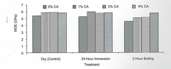
Figure 3. Column chart of modulus of elasticity (MOE) in relation with the different treatments of coupling agents (CA) for sisal fiber plastic composites
