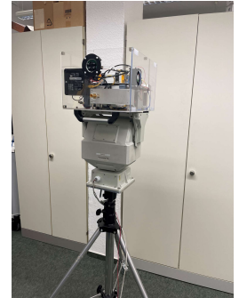
Figure 2: Picture of the TX quad-band channel sounder
