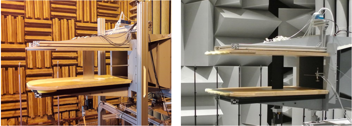
Figure 2.1: View of the experimental setups: (a) first campaign with NACA 0012 airfoil (b) second campaign with NACA 633418 airfoil.
