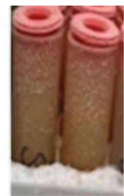
Example of cryovial that has been overfilled with more than 1mL of serum. Note that the caps are no longer secure.
