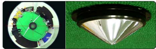
Fig. 4 The hyperbolic mirror and the typical panoramic image captured
