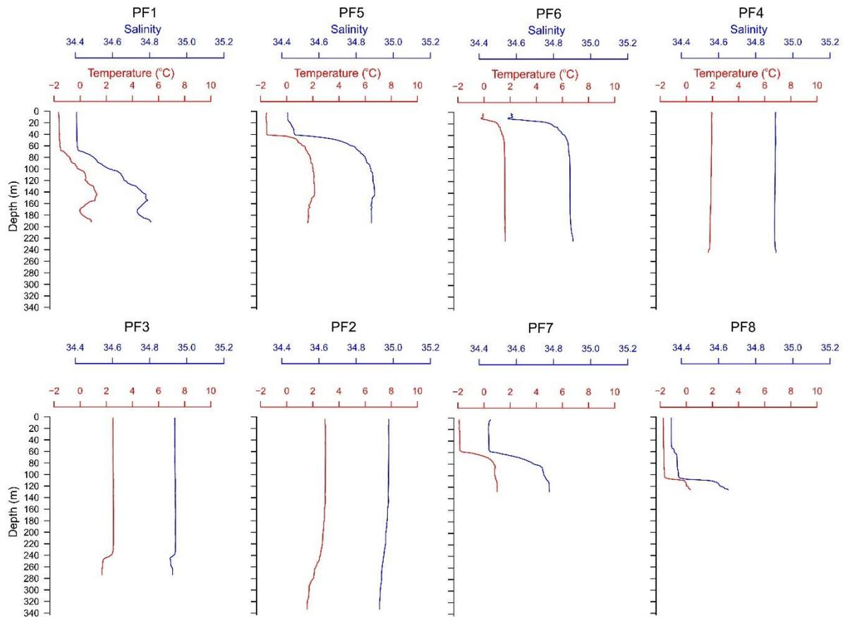
**Figure 4:** CTD profiles at full stations taken with Seabird 911 on the Helmer Hanssen rosette. Stations PF1-6 are ordered from north to south (see Figure 1), PF7 and PF8 were located west of the main transect. Data are not quality controlled.
