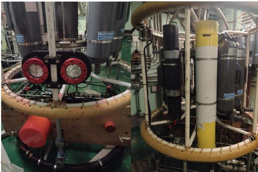
*Figure 4.9.1. Installation of the WBAT and light system (Fish Disco) on the Rosette (Image from previous survey in January 2023).*
