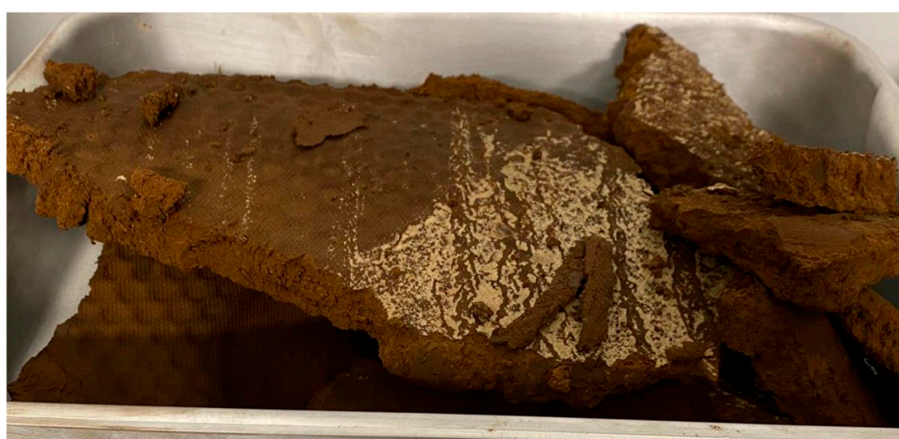
Figure 2. Wet press cake obtained after dewatering of the product slurry after carbonization of olive pomace.
