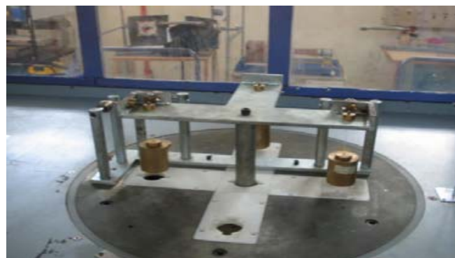
Fig.4. Calibration rig mounted on the wind tunnel test section
