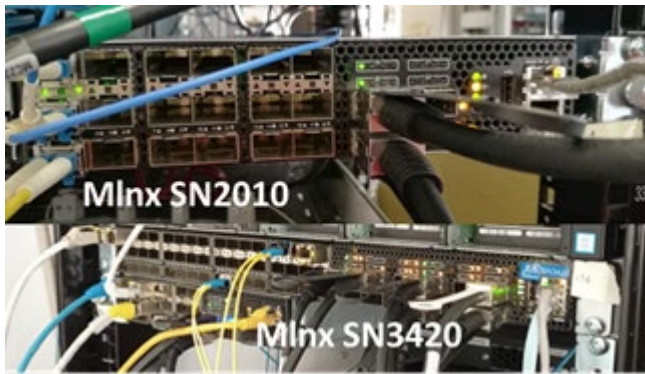
FIGURE 44. ARNO: AGGREGATION SWITCHES
