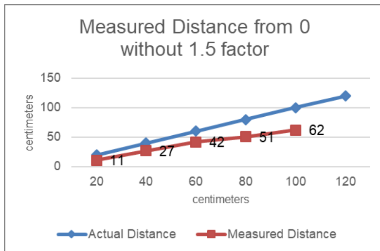
Figure 3.3.8: Test 2 - Measured Distance from zero without 1.5 correction factor for single UE transmit antenna
