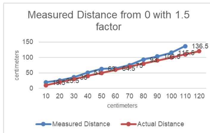
Figure 3.3.32: Test 2 with absorbers - Measured Distance from zero with 1.5 correction factor for single UE transmit antenna
