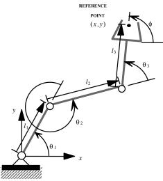
Fig. 2 Three link manipulator
