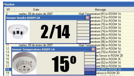
Fig. 8. Temperature Sensor, Smoke Sensor and Monitor Screens.
