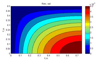
Fig. 8 Rotation around x-axis of non-optimized plate
