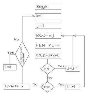
Fig. 1 The optimization algorithm
