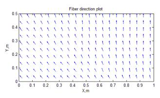
Fig. 3 The plot of fiber directions in each finite element of quarter of optimized plate with dimensions 1.0(m)x2.0(m)
