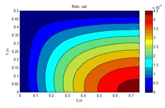
Fig. 9 Rotation around x-axis of optimized plate
