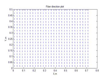
Fig. 2 The plot of fiber directions in each finite element of nonoptimized plate with dimensions 1.0(m)x1.5(m)
