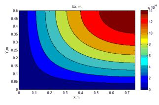
Fig. 6 Transversal displacements (m) of non-optimized plate
