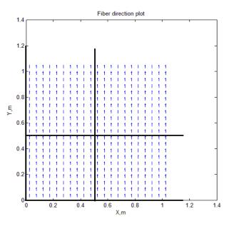
Fig. 10 The plot of fiber directions in each finite element of nonoptimized three span plate (shown quarter of plate), bold lines indicate vertical supports
