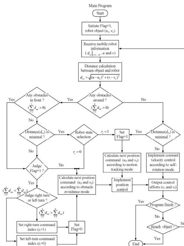
Fig. 2 Main flow chart of adaptive path-planning control
