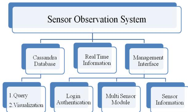
Fig. 4 The architecture of sensor observation system
