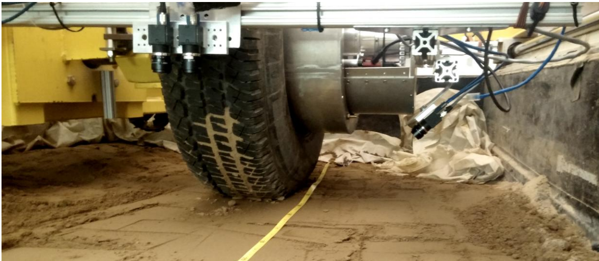
Fig. 3. Complete system undergoing testing in the terramechanics rig at Virginia Tech. Visible in the top left are the cameras responsible for measuring the profile in front of the tyre
