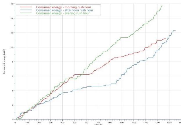
Fig. 5. Electric Bus model – Consumed energy evolution
