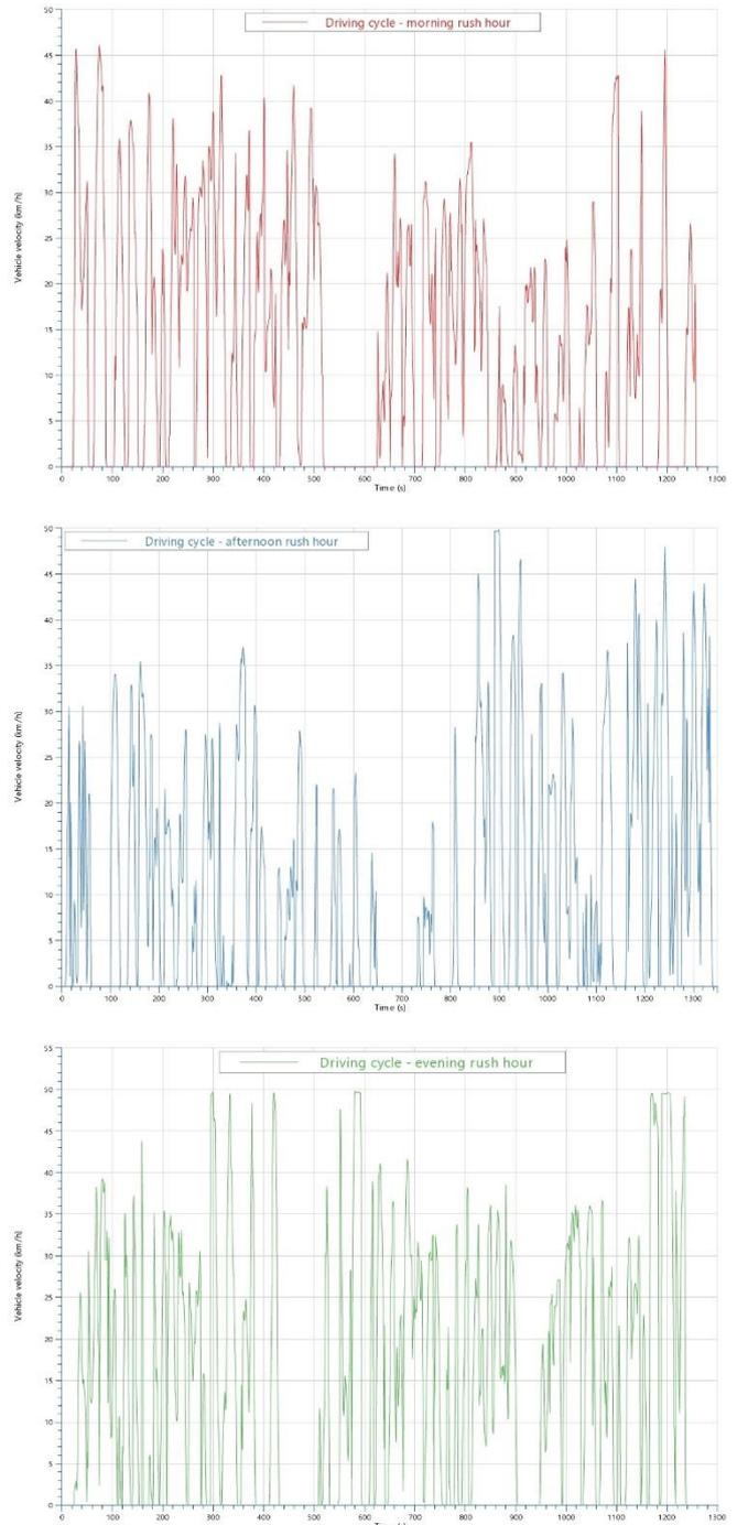
Fig. 3. Simulated driving cycles – morning rush hour (top), afternoon rush hour (middle), evening rush hour (bottom)
