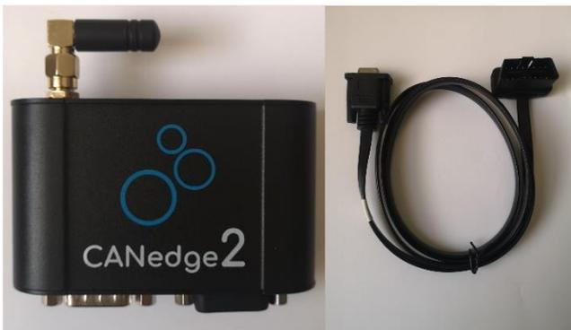
Fig. 2. CANedge2 device used for bus data collection
