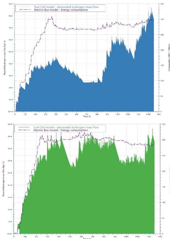
Fig. 9. Comparison – Demanded hydrogen mass flow vs Energy consumption – Afternoon rush hour (top), Evening rush hour (bottom)
