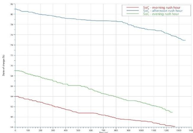
Fig. 4. Electric Bus model - State of Charge evolution
