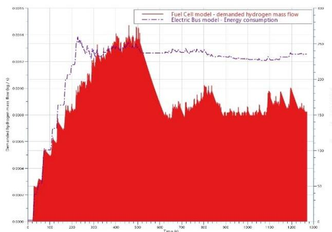
Fig. 8. Comparison – Demanded hydrogen mass flow vs Energy consumption – Morning rush hour
