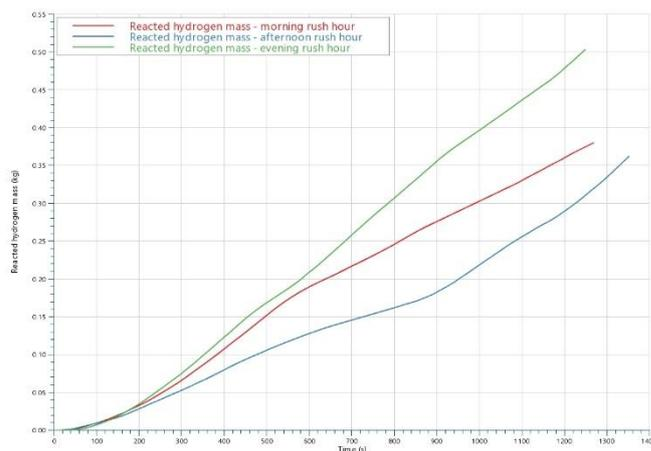
Fig. 7. Fuel Cell Bus model – Reacted hydrogen mass evolution
