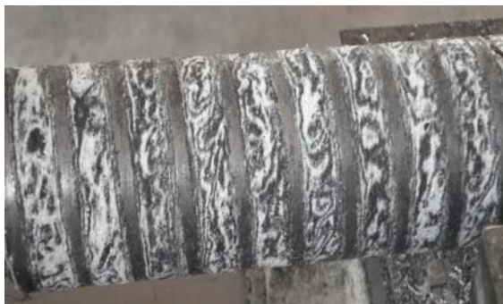
Fig. 3 Fibers wound on the mandrel
