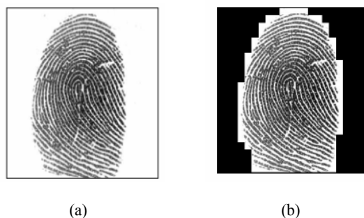
Fig. 2 Foreground segmentation (a) Original image (b) Segmented image
