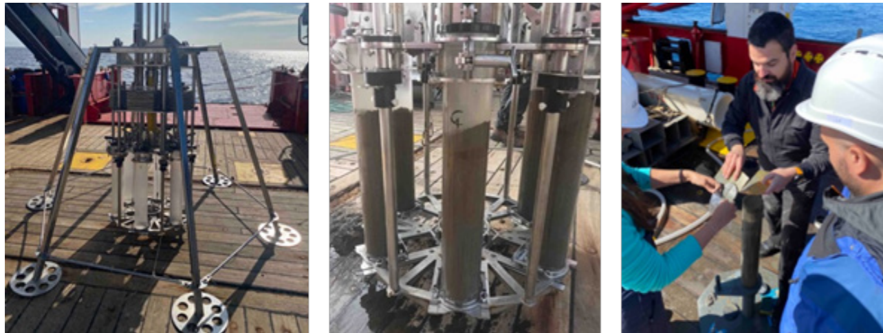
Figure 25. Multicorer system used during FARDWO-DS1 cruise and an example of sediment recovery and sampling.
