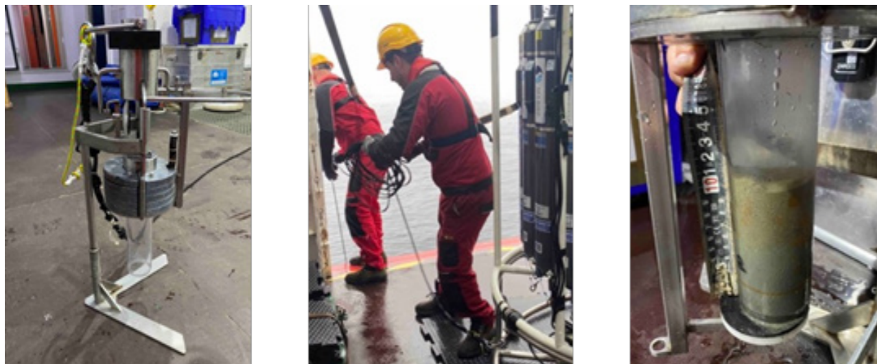
Figure 22. Monocoher system, deployment operation and sample recovered in FDDS1_009_MoC station.
