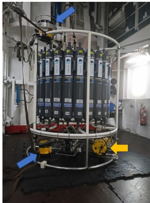
Figure 9. Locations (blue arrows) of the upward and downward looking ADCPs installed in the CTD-rosette ensemble. The external battery canister is marked with an orange arrow.
