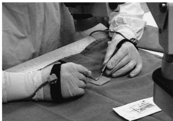
Fig. 1 Electromagnetic trackers placed on backs of microsurgeons' hands allowed positional data to be recorded and analyzed by computer software while subject performed a standardized microsurgical task [9]
