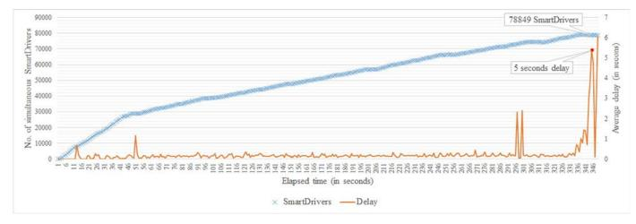
Fig. 14. Kafka configuration 3 using servers type 2. This setting uses 6 brokers per node.
