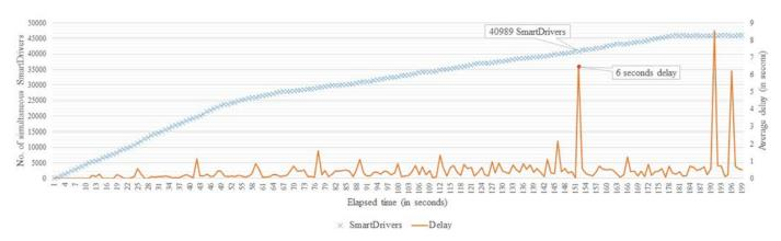
Fig. 13. Kafka configuration 1 using server type 2. Incrementally increasing simultaneous SmartDrivers and delay detected.
