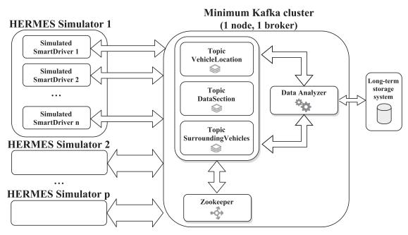
Fig. 8. Kafka configuration 1: Minimum Kafka cluster consisting of only one node with one single broker.
