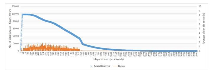
Fig. 15. Kafka configuration 4 using servers type 2. This setting uses 8 brokers per node. Full-size trace of best result achieved covering almost 100,000 simultaneous SmartDrivers.
