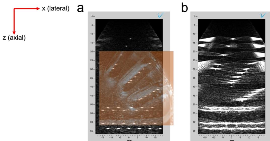
A Verasonics acoustic plane wave simulation of 128 transmit and 64 receive channels with acoustic scatterers was placed in areas where cavitation was predicted to occur. Acoustic scatterers are placed in the **(a)** sulci and central sulcus regions, revealing **(b)** high-intensity regions in the lateral direction.
