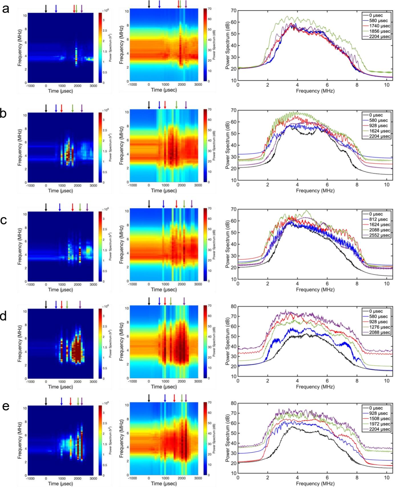
Acoustic spectral analysis regarding averaged 64 channels revealing linear and log power spectrograms and time-dependent logarithmic spectra. The following tests involve a better sealing method and go as follows: **(a)** of a single-layer brain phantom, **(b)** a two-layered phantom, and **(c)** DI water. Both tests regarding **(d)** a two-layered phantom and **(e)** DI water correspond to tests with more pre-existing bubbles.
