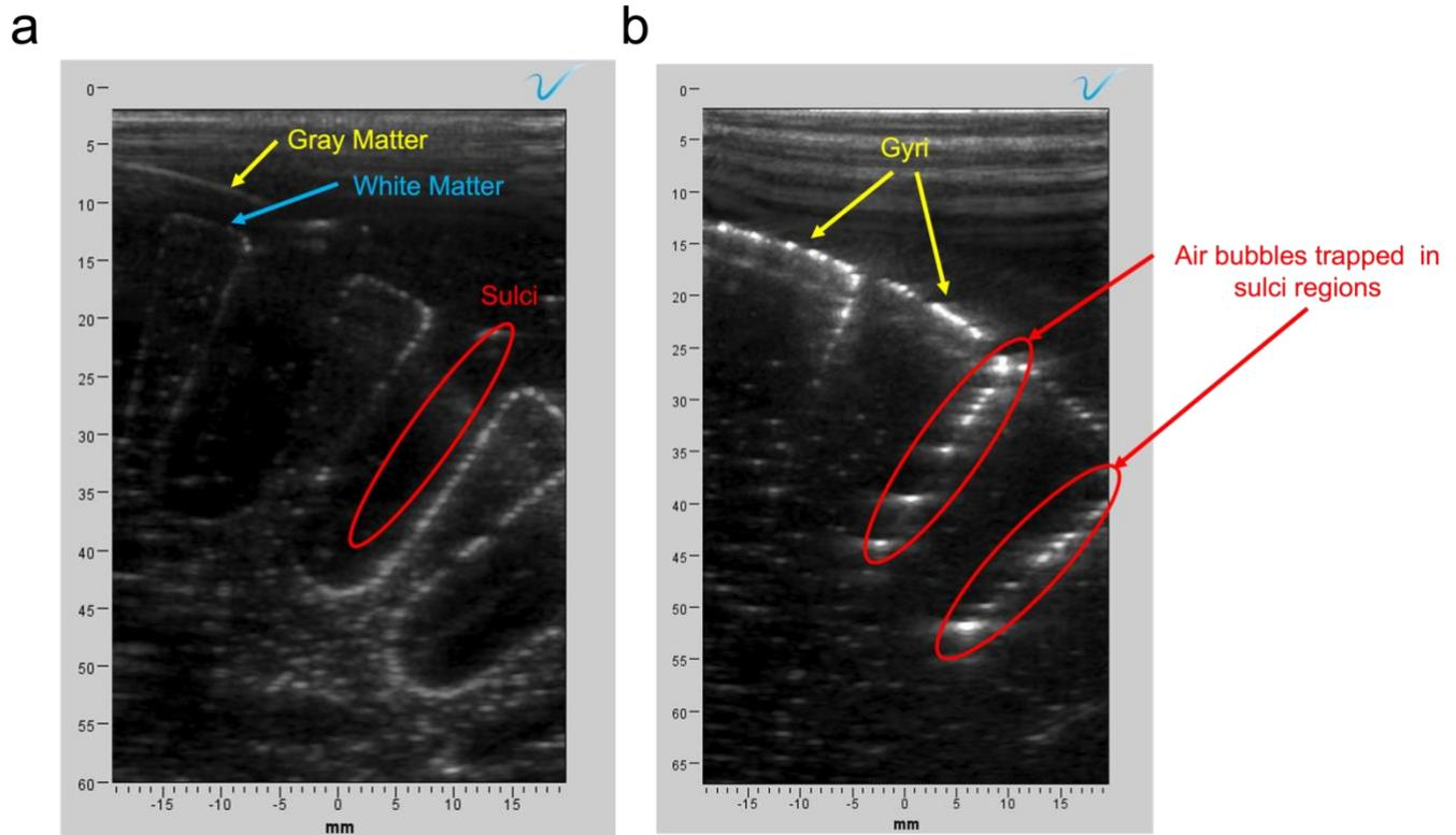
A high-quality wide-beam image of a (a) two-layer brain phantom reveals the gray and white matter where the interface is illuminated as high-intensity regions from trapped pre-existing bubbles during the polyacrylamide polymerization process. A (b) single-layer brain phantom displays trapped air bubbles in the sulcal regions after swelling for more than 24 hours in an isotonic solution. Both acoustic images were taken before impact and are caused by sealing and hydrogel fabrication methods.
