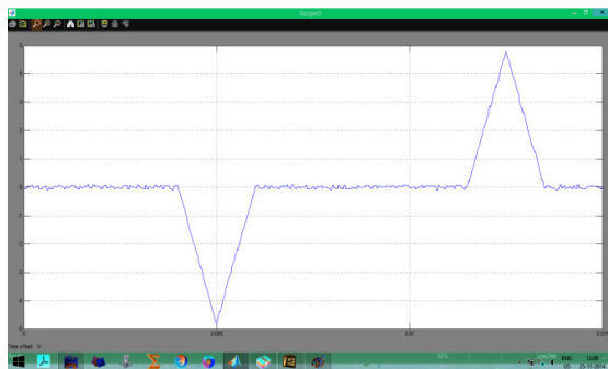
Fig.5.6.4 Estimation of load current i_c by the RMP model
