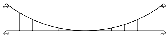
Fig. 4 Suspension bridge stabilization by connecting of main cable and girder at the centre of span
