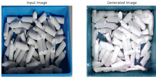
Fig. 5: Image before CycleGAN (input synthetic image) and after (generated image)
