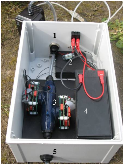
Fig. 3 Internal layout of System I
