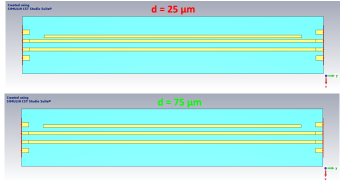
Fig. 8. Investigated configuration of asymmetrical adjacent structures.
