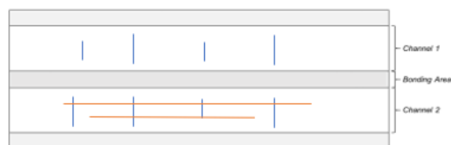
Figure 10 –Type of the scanning lines performed, vertical (blue line) and longitudinal (orange line).
